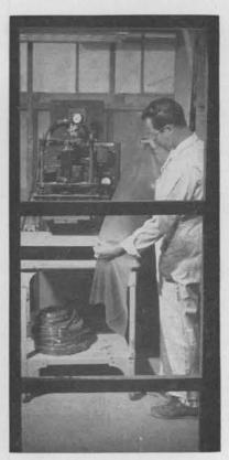
MICROWAVE PRESS welds seams in vinyl film. Kenneth L. Peterson operates the machine which generates heat through molecular action in material.
